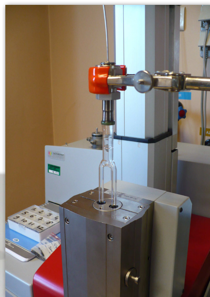
Figure 12 – Silica glass finger and the adaptation to the CALVET PRO DSC
