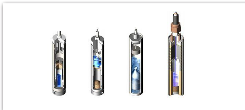
Figure 1 – Some of the most typically used calorimetric mixing cells (from left to right: reversal, membrane, ampoule and percolation mixing)
