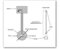
Schematics of the setup after microbalance integration (reproduced from [1])
