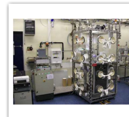
High temperature calorimeter placed in a glovebox (reproduced from E. Capelli et al. / J. Chem. Thermodynamics 58 (2013) 110 -116)
